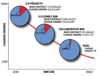
Figure 1. BIM use and change order comparison.
